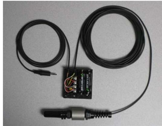
In this final step, the hydrophone and output cables will be prepared and connected together along with the remaining components within the battery/terminal enclosure.
