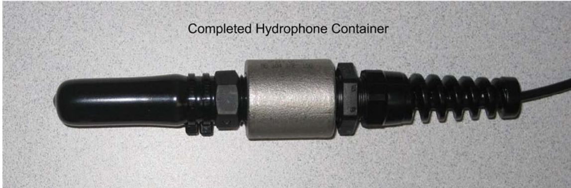
The hydrophone container is the underwater component of the system designed to provide a watertight enclosure in which to house the microphone element. In this design, the hydrophone container utilizes simple nylon and stainless steel parts that seal to one another by means of compression.
