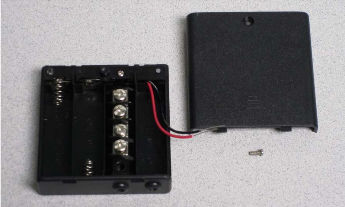
The battery/terminal enclosure provides a single, splash-proof environment for the provision of power to the hydrophone as well as for connections between the hydrophone cable and the output cable. The basis for this enclosure is a simple 4 “AA” on/off battery holder that you will modify to accommodate the required 2 “AA” batteries and terminal block, necessary to make the final connections.
